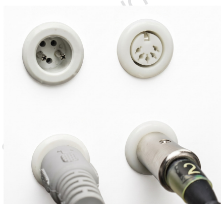
FIGURE 14 Sockets on the unit and their connectors: each cable goes into its own socket, respecting the numbering.
