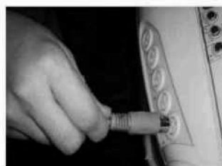
FIGURE 15 Connection of the infrared heating circuit.
